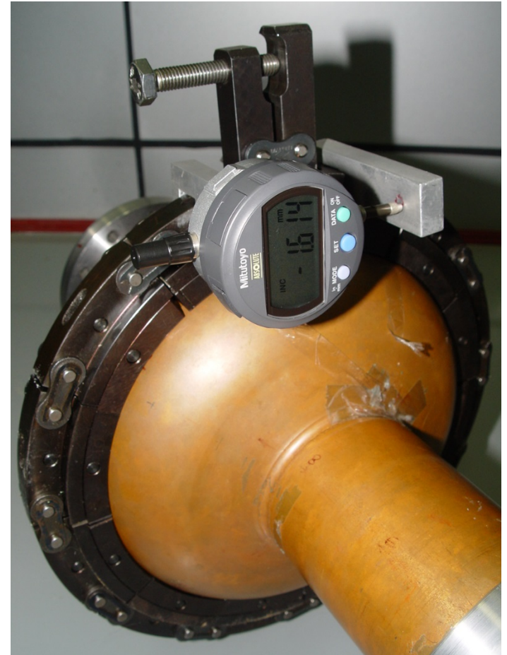
Chain Link Tuner mounted on single cell cavity
