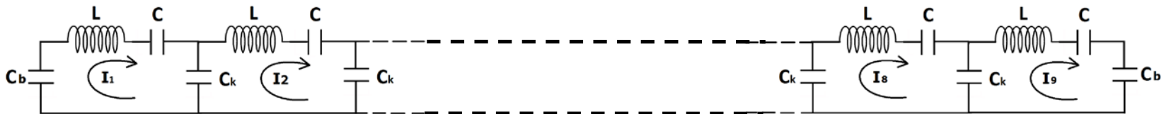
Equivalent circuit of a 9-cell SCRF cavity
