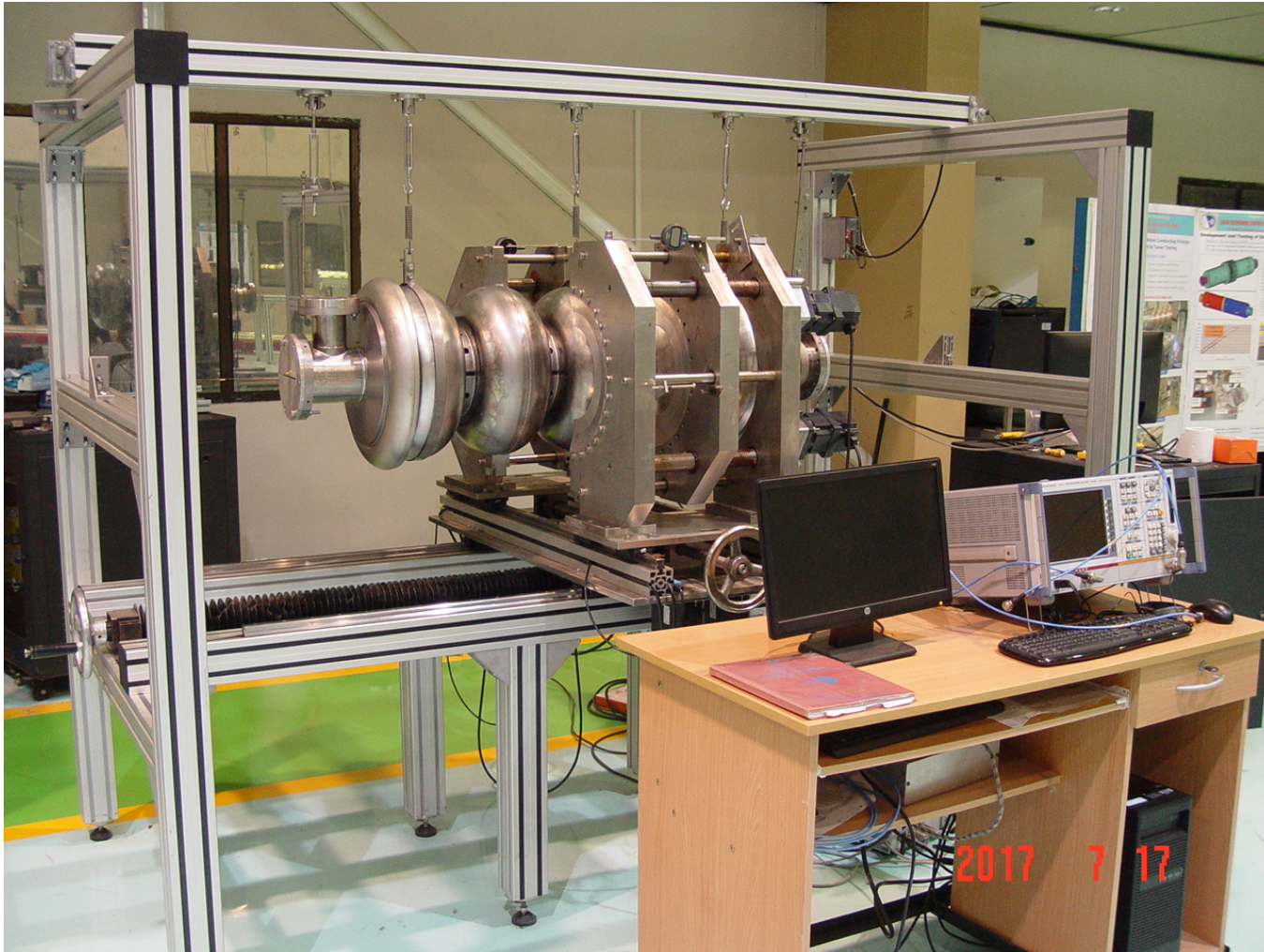
650 MHz \beta 0.92 Five Cell SCRF cavity mounted machine for tuning operation
